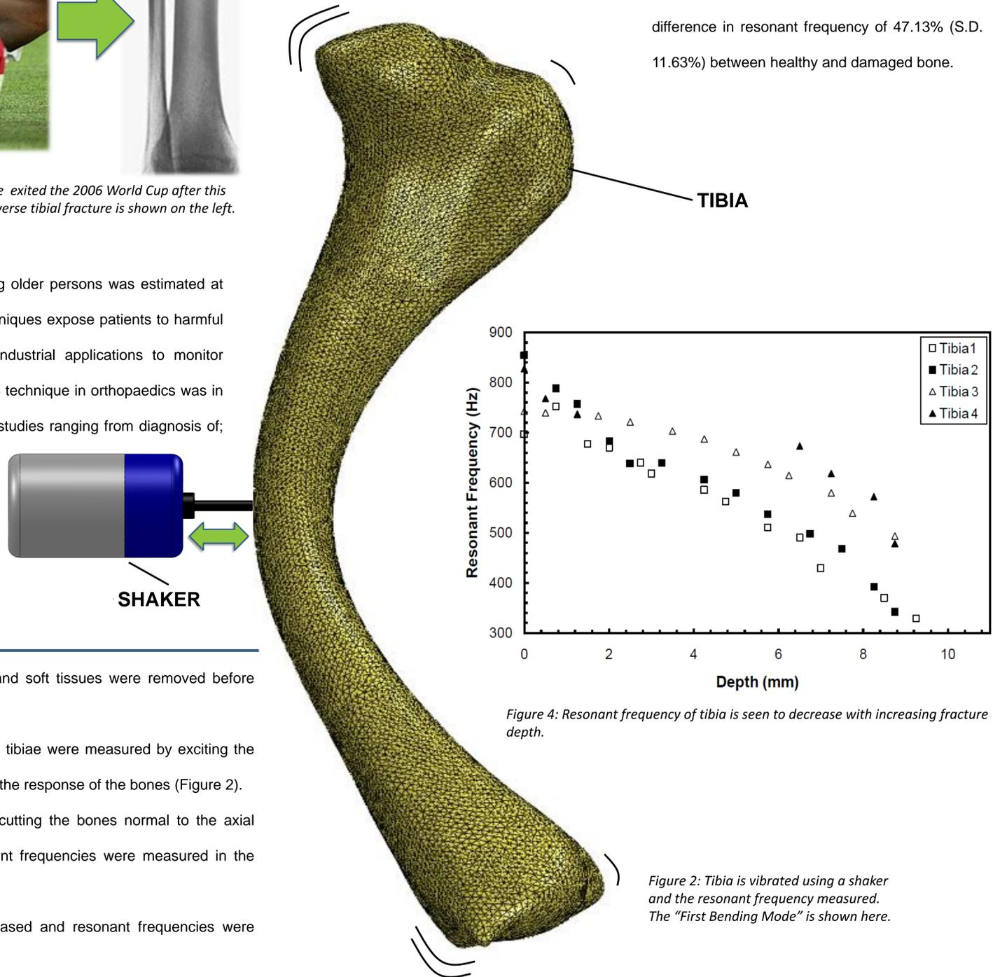
Figure 4: Resonant frequency of tibia is seen to decrease with increasing fracture depth.
