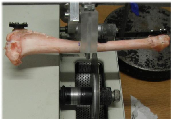
Figure 3: A fracture is simulated by cutting the tibia at the mid-diaphysis using a low speed saw.
