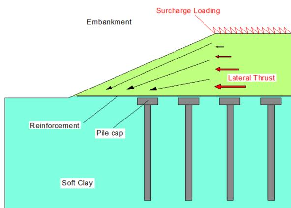
Figure 1. Reinforced pile embankment
