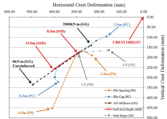
Figure 4. Relationship of crest deformation for a range of parametric variations
