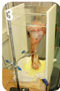
3.) The bones were then clamped in position and one end was moulded in dental cement at a time using a custom built rig which was capable of shaping the mould and orientating the bone in a replicable manner.
