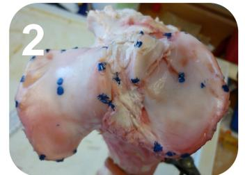
2.) The tibiae were then marked out to find the centres of the articulating surfaces in order to orientate the bones in a replicable manner for moulding.
