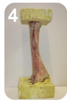
4.) The bones were then extracted from the mould rig and covered in vaseline to preserve the water content in the bone for the duration of the test.
