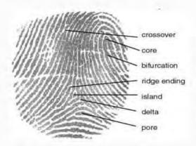
This fingerprint shows what the fingerprint scanner is looking for when running a scan. No two fingerprints are fully identical; This is why when the finger is scanned; the scanner picks up on multiple parts of the finger to make that sample unique.
