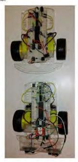
A mobile application can communicate with the lead vehicle to stop, pause or reset the demonstration while in the process displaying the Platoon speed.
