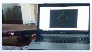
This skeletal program is then opened in Visual Studio where thresholds are set to indicate where the users hand is, this data is then used along with an Arduino sketch that is imported to Visual Studio that will take in the commands of the Kinect. It will then be sent over Bluetooth from the laptop to the HC-06 which will then indicate to the Arduino Nano and L298N driver which motors on the chassis will move.
