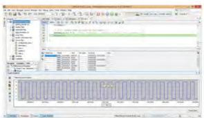
Each program instruction cycle time is accounted for using the Analyser and Special Function Registers view of MPLAB X
